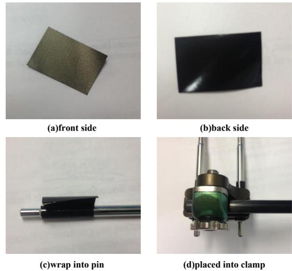
Fig. 10 setup for absorption material
