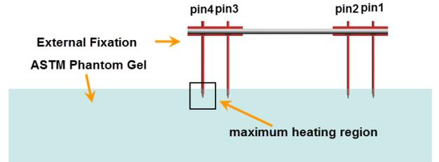
Fig. 4 Side view of external fixation geometry
