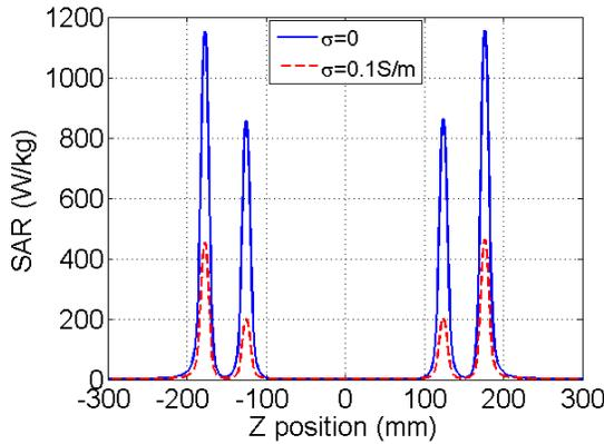
Fig. 6 SAR along green line that across the tips of pins ( $\epsilon_r=9$ )
