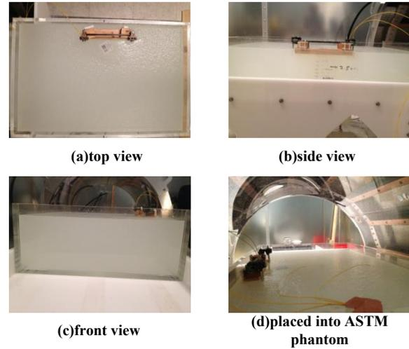
Fig. 9 Experimental setup for external fixation and ASTM phantom
