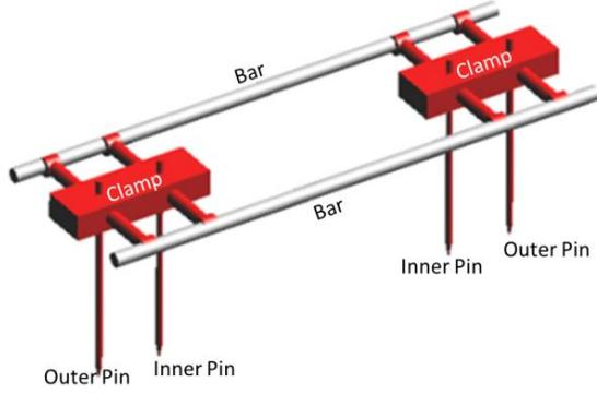
Fig. 1 Typical structure of external fixation devices
